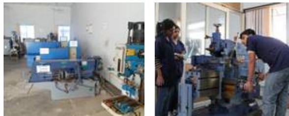
**Manufacturing Laboratory:** The Manufacturing Laboratory has facilities such as lathes, milling machine, vertical machining centre, electric discharge machine, welding, fitting and tin smithy equipment. It supports courses on Manufacturing Practices and Processes and for supporting manufacturing activities in Integrated Design and Manufacturing courses. It also serves as a workshop for fabrication of undergraduate student projects as well as research related equipment and accessories.
