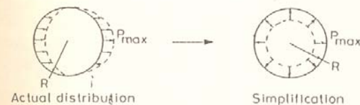
(a) Simplified hydrodynamic pressure distribution on tank wall
