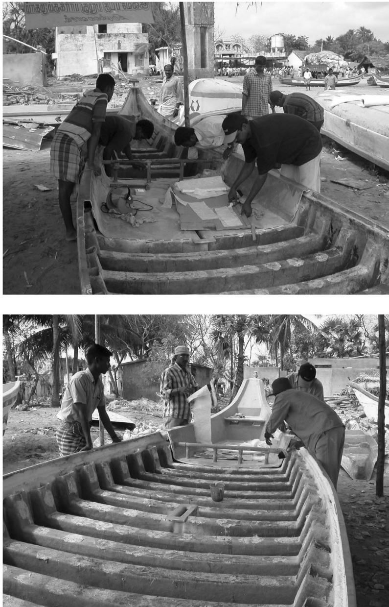
Figure 9. Repairmen from Kerala working in the Nagapattinam area to fix fiberglass boats for redeployment.
