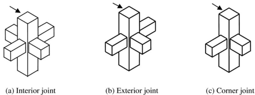
Fig. 1 Types of joints in a moment resisting frame
