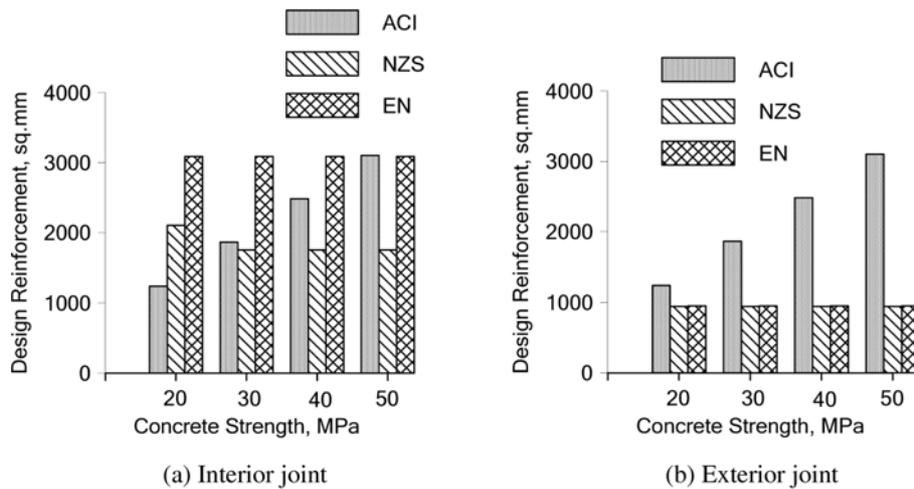
Fig. 9 Effect of concrete strength on design shear reinforcement
