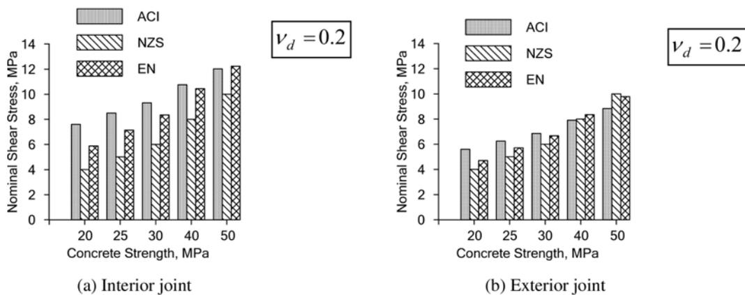
Fig. 7 Effect of concrete strength on nominal shear stress
