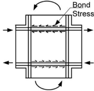
Fig. 2 Bond condition in an interior joint
