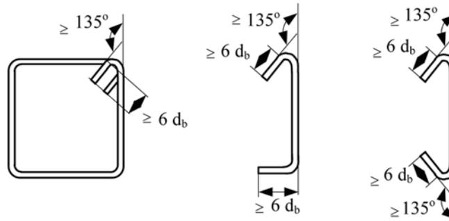
Fig. 11 Typical configurations of stirrup and cross-ties
