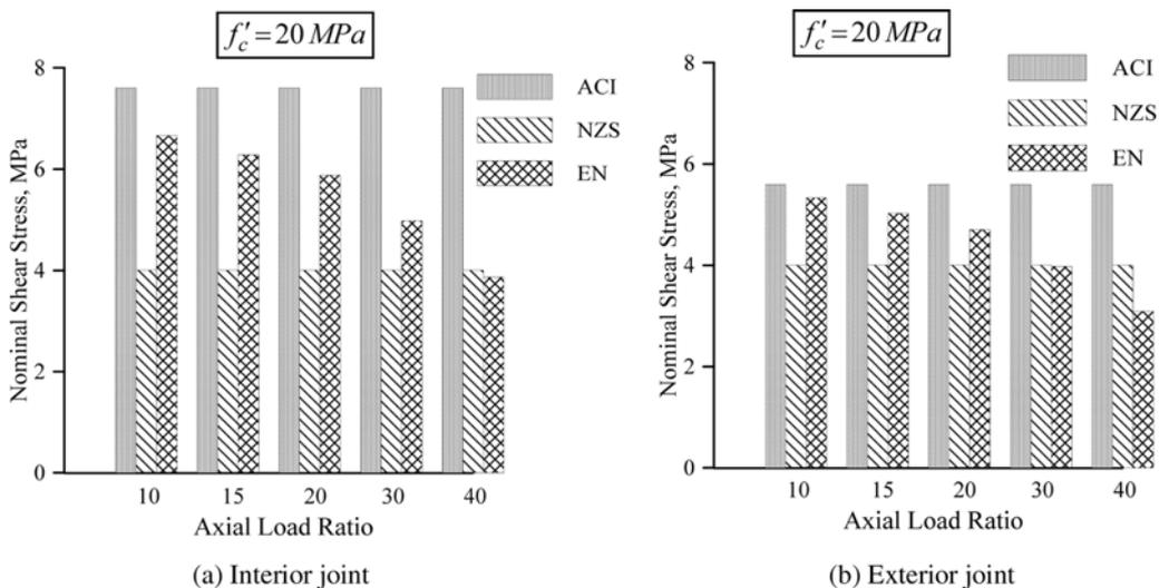
Fig. 8 Effect of axial load on nominal shear stress
