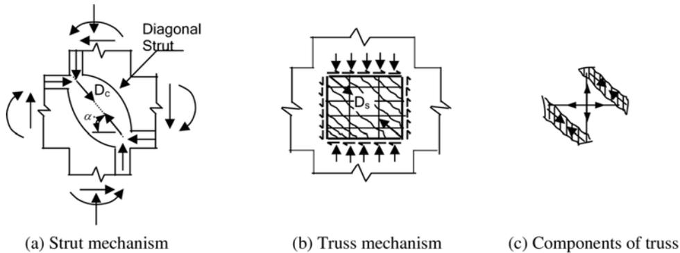
Fig. 6 Shear resisting mechanisms
