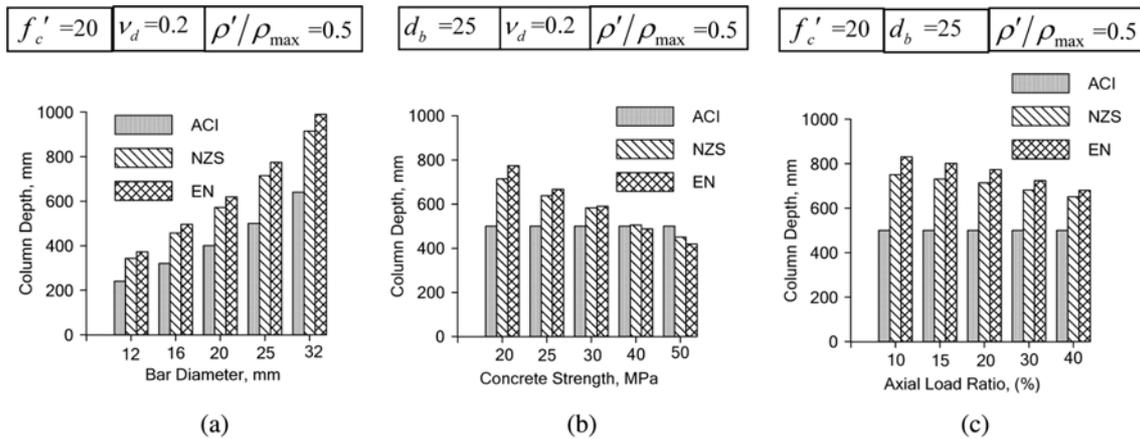
Fig. 3 Variation of column depth for interior joint
