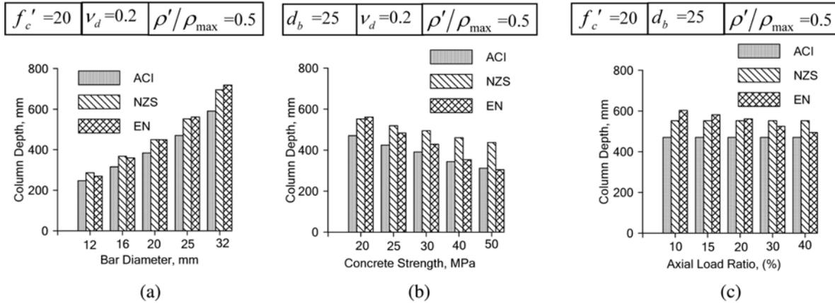
Fig. 5 Variation on column depth for exterior joint
