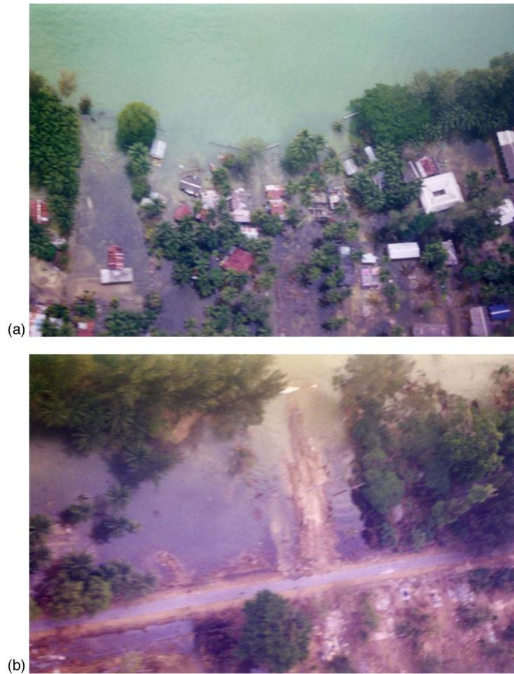
**Figure 6.** (a) Inundation and submergence of the area along the eastern coastline of Great Nicobar Island because of subsidence caused by the 26 December earthquake. (b) A coastal road encircling the island was damaged and submerged due to subsidence (photos: J. Malik).
