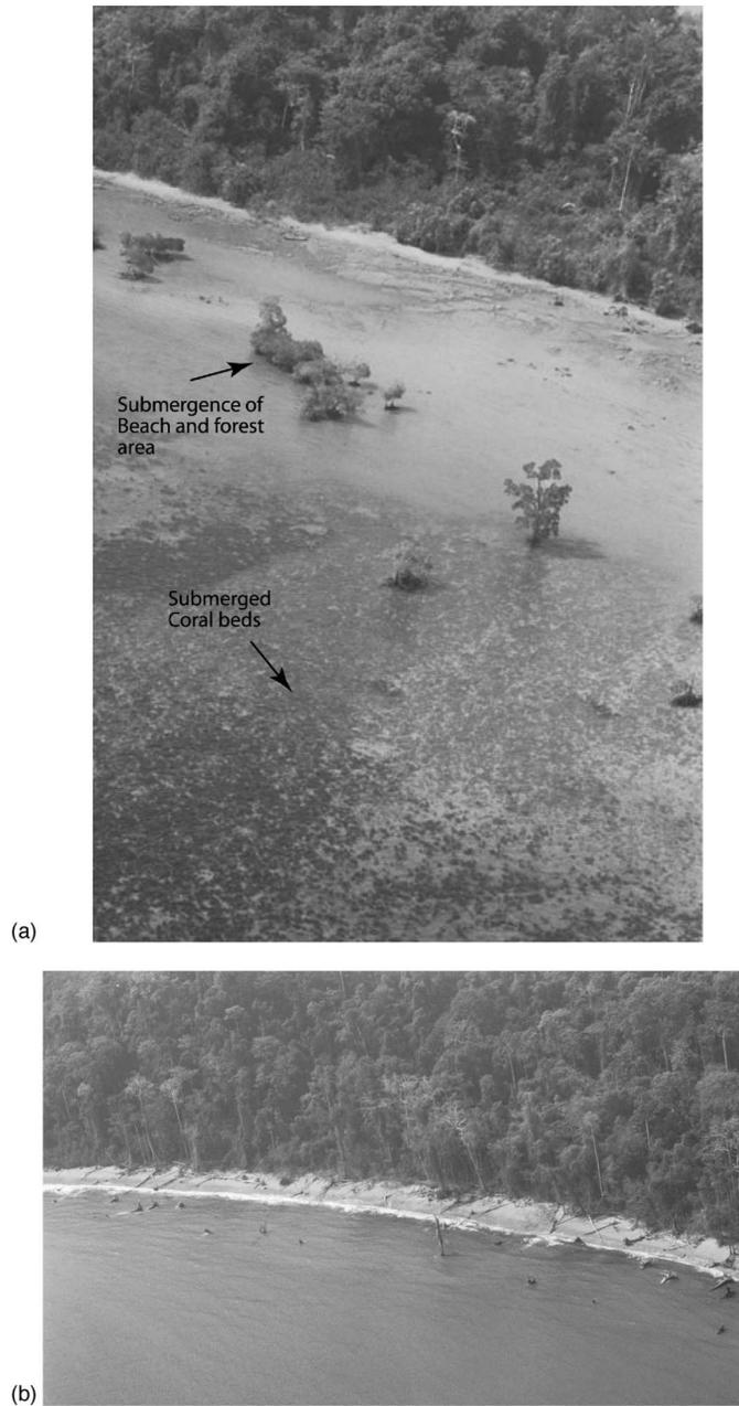
**Figure 16.** (a) Submerged coral beds, beach, and forest area along the eastern coast of South Andaman Island near Baratang Island. Submergence is due to tectonic subsidence of the east coastline as a result of the 26 December earthquake. (b) Submerged coastline and dead trees along the western coast of Middle Andaman Island (photos: J. N. Malik).
